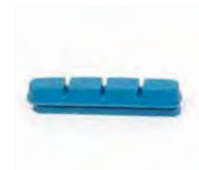
6827 -CARD Road Compatible with Shimano 55 mm replacement pad for 6833, 6835, 6845, 6847 For carbon rims only
